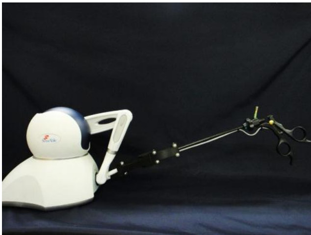
Fig. 2. Haptic Device for Master-Surgical Robotic Controlling [13].
