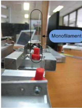
Figure. 8. Monofilament when being as a part of the Robotic Monofilament Probe.
