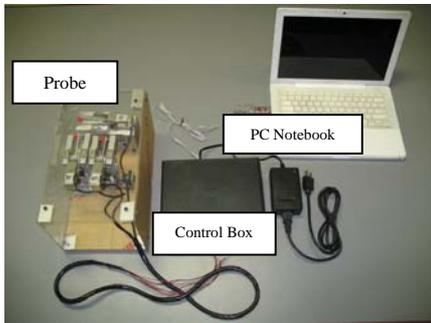
Figure.9. System of the prototype “Robotic Monofilament Probe”
