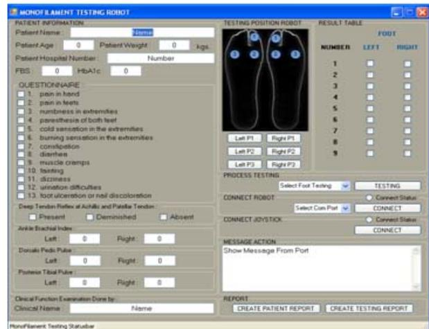
Figure 5. Graphical User Interface (GUI) for command and control Robotic Monofilament Probe, and also collect patient's information and test result.
