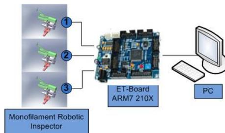
Figure 6. Control Box to control an action of Robotic Monofilament Probe.
