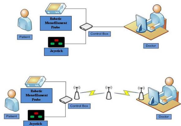
Figure 3. System diagram: GUI and Controller Command, Control box, and Robotic Monofilament Probe.
